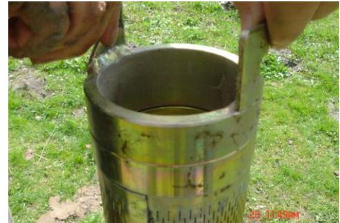
An approximation of the permeability factor may be made by classifying the soil removed from the hole based on the average grain size (See table 1).
