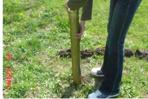
➔ **In a sandy soil a filter is inserted into the hole to prevent the walls of the bore hole from collapsing.**
