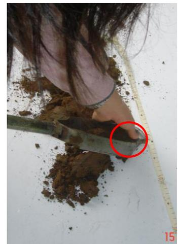
Make a soil profile of the bore hole.
