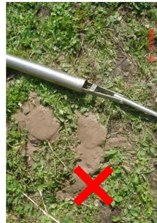
Do not overfill the auger. In clayey soils this will cause severe smearing of the borehole wall and reduce permeability greatly.
