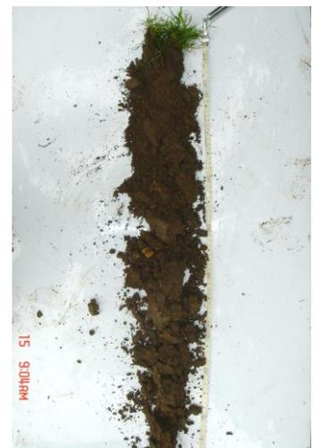
The minimum drop in water level you should be able to create is 20 cm. This means that the auger hole should have a minimum depth of 25cm under the groundwater level (preferably 35cm). A deeper hole will facilitate the bailing out of water and increase the volume of soil in which you are measuring so of which you are determining the permeability.
