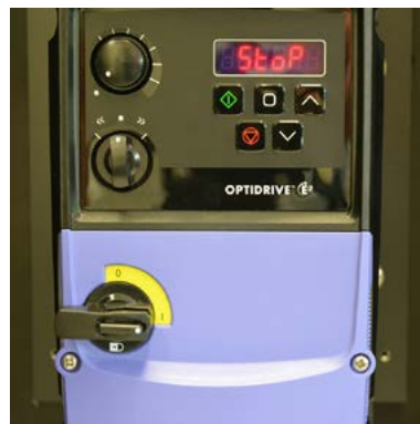
Fig. 8b Switch 1 set to ON
