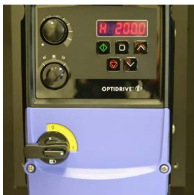
Fig. 8d Switch 3 set to 200 Hz
