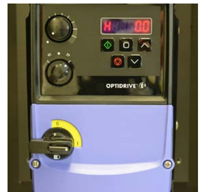
Fig. 8c Switch 2 set to >> forward
