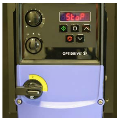
Fig. 8b Switch 1 set to ON
