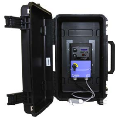
Fig. 7 Vertical installation of the converter
