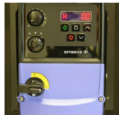
Fig. 8c Switch 2 set to >> forward
