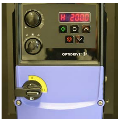
Fig. 8d Switch 3 set to 200 Hz
