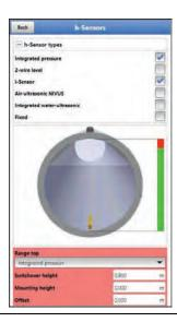
Fig. 39-9 Selecting sensors and display of sensor measurement ranges
