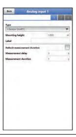
Fig. 39-25 Analogue input as External Measurement Value / i-Sensor (HART)
