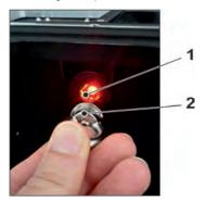
Fig. 31-10 Waking up the NivuFlow Mobile
