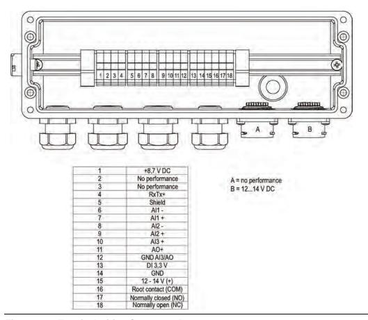
Fig. 27-2 Terminal wiring Connector Box
