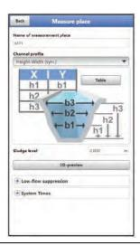
Fig. 39-4 Setting profile parameters using Height-Width (sym.)
