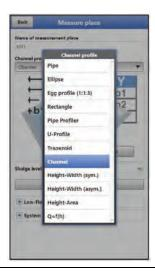
Fig. 39-2 Selectable Channel Profiles
