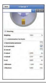
Fig. 39-21 Submenu: v-Determination low Levels
