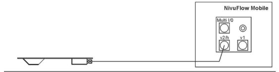
Fig. 25-2 Connection of DSM-L0 level sensor
