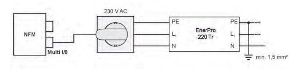
Fig. 25-5 Overvoltage protection for power supply AC general
