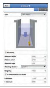
Fig. 39-18 Entering the Sensor Position, relative to the Application Centre
