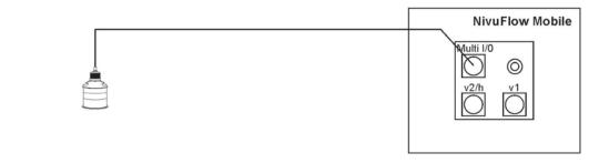
Fig. 25-3 Connection of i-Series and NivuBar Plus level sensors
