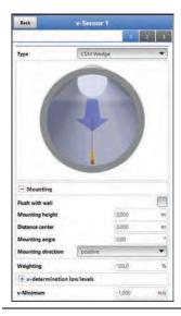
Fig. 39-14 Setting Parameters using Height, Distance and Angle
