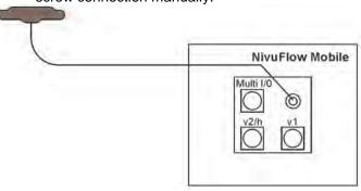
Fig. 28-1 Connecting the 2G/3G/4G antenna
