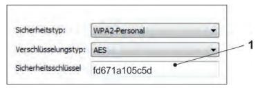
Fig. 31-22 Enter security key and connect
