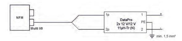
Fig. 25-6 Overvoltage protection for power supply DC general
