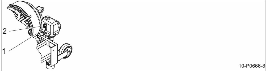
Fig. 13 Checking pressure relief valve on the air receiver
