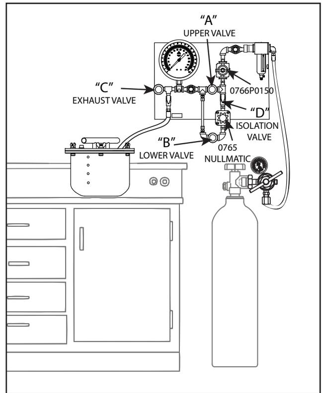
(Fig.06) Lab053 - Nitrogen as a Pressure Source
