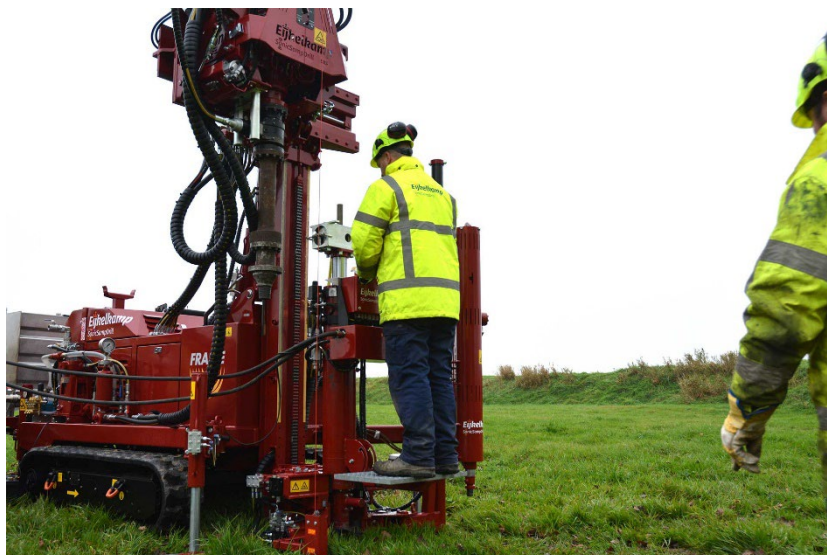
Figure 2: Performing CPT with a drill rig a cost-effective way to explore CPT
