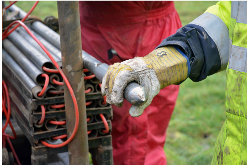
Figure 1: CPT is performed with a cone attached to a string of rods
