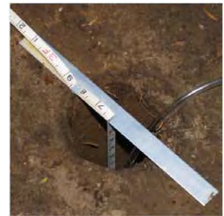
Fig. 19. Tape secured using Tape Holder.
