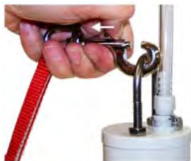
Fig. 15. Connecting Tape Hook to RU.
