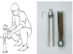
5. After locating the intended spot, press the auger vertically into the ground to the desired depth. If necessary an impact absorbing hammer can be used to drive the auger into the ground.
