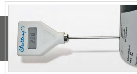
The functionality can be tested directly on the instrument quickly and simply using the optional attachment unit
