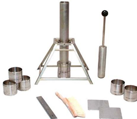
The core cutter method (Dutch RAW-standard 2010, Test No. 6) is used to determine the density and moisture content of embankment or foundation materials (in situ method).
