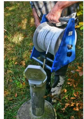
Water level meters are part of the standard equipment for the ascertainment of ground water levels. These mobile units are characterised by their simple, fast and solid acquiring of water level. With the variety of available models, you have the possibility to select the appropriate unit according to your individual requirements in cable length or operating convenience.
