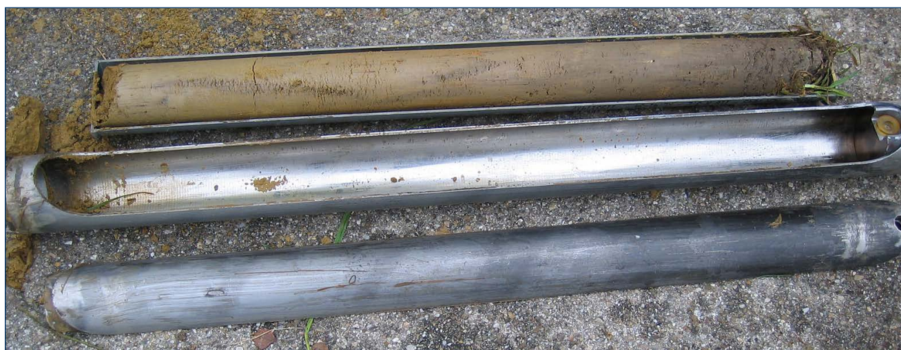
Soil column cylinder, removable lid and sample in sample gutter
