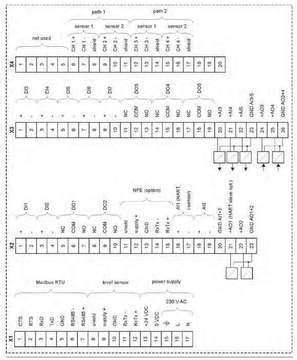
Fig. 21-5 Terminal connections NivuFlow 650 Type TR
