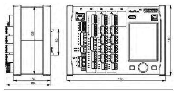
Fig. 15-2 Dimensions of NivuFlow 650 enclosure type E0
