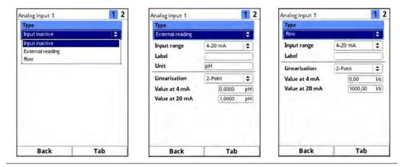
Fig. 32-16 Analog inputs: Activation / Ext. Reading / Flow
