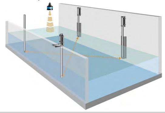
Fig. 28-1 Application example: rectangular channel with 2 measurement paths
