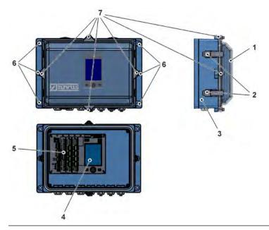
Fig. 20-1 Fastening the field enclosure
