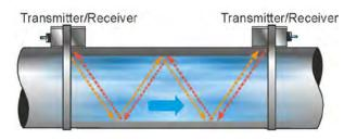
Fig. 22-3 Example "Diametral W" mode
