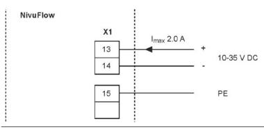
Fig. 21-8 DC connections of power supply
