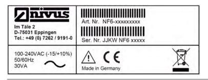
Fig. 15-4 Nameplate AC version
