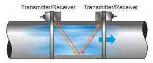
Fig. 22-2 Example "Diametral V" mode
