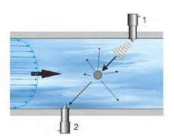
Fig. 18-1 Signal damping by interfering particles
