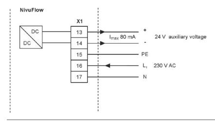
Fig. 21-9 AC power supply wiring
