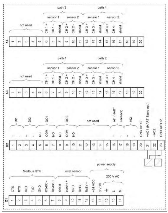
Fig. 21-4 Terminal connections NivuFlow 650 Type T4
