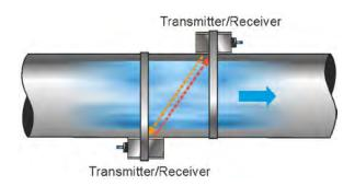
Fig. 22-1 Example "Diametral \" mode
