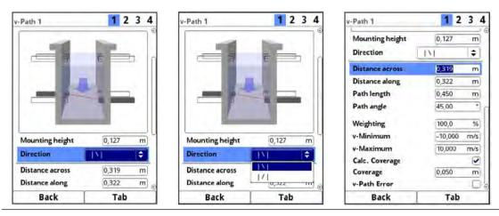
Fig. 32-13 Sensor mounting
