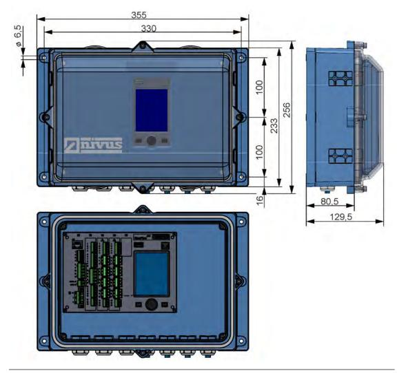
Fig. 15-3 Dimensions of field enclosure NivuFlow
