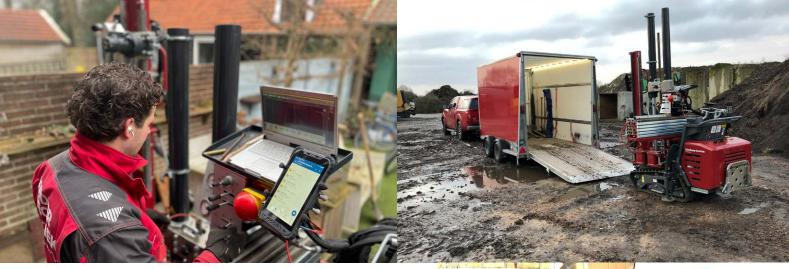
'The Compact Crawler CPT 200 is compact and, by being well anchored, very powerful. And that is quite special for such a small machine. Anchoring takes some time, but you can get anywhere with it, like indoor and backyards.'
