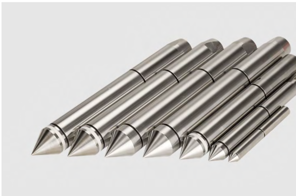
Figure 5: CPT cones ranging in size from 15.2 cm 2 to 2 cm 2
