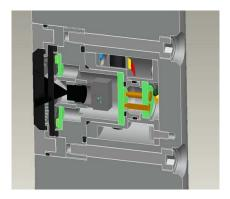
When removed you will find four screws (on every corner). Unscrew to remove top cover with sapphire glass and o-ring. Replace with new glass and screw assembly together. Please ensure to put o-ring back in the right way to prevent the probe to leak water inside.
