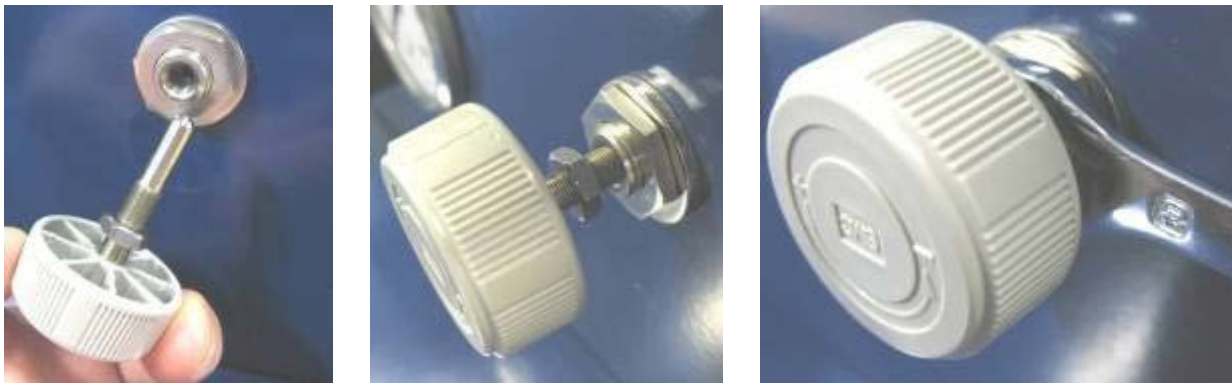
Fig. 17 Tightening the nut of the needle regulator slightly
