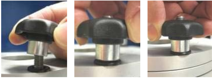
7a. 7b. 7c. Fig. 7 Fixing the clamp ring using special 'fast screwing nuts'
