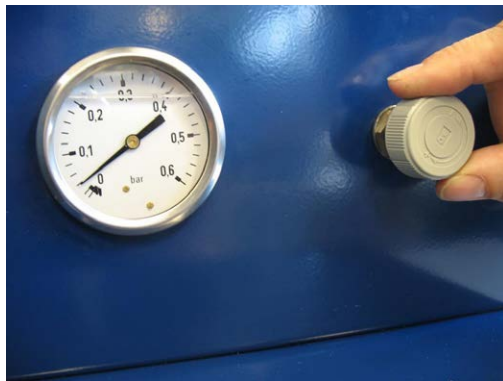
Fig. 10b Regulate the air pressure
