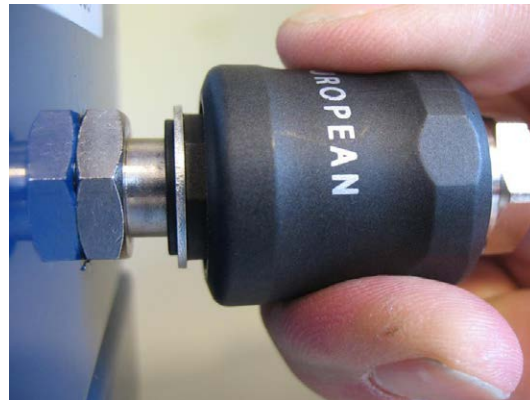
Fig. 2b Firmly push the coupling onto the connection
