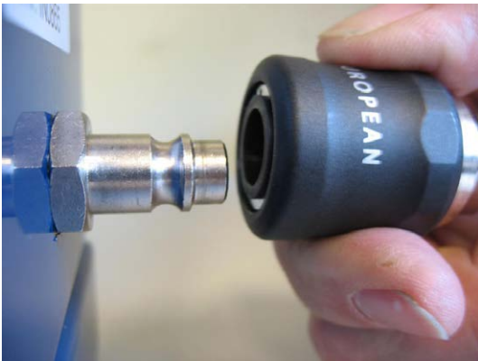
Fig. 2a To connect the air supply
