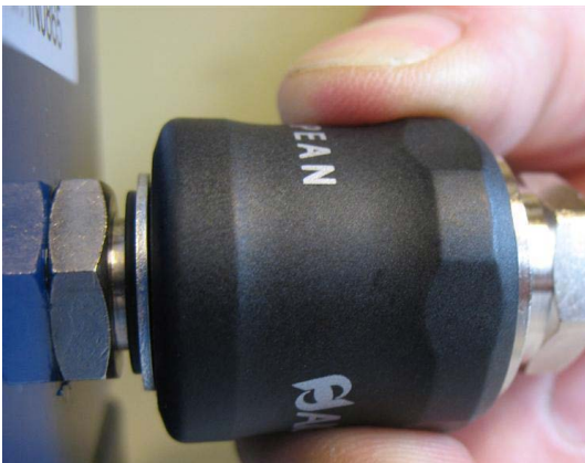
Fig. 3a To release: pull back the black ring
