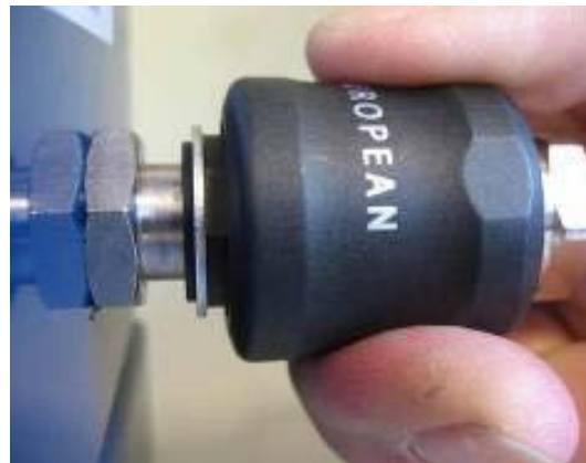
Fig. 3b Pull further to disconnect
