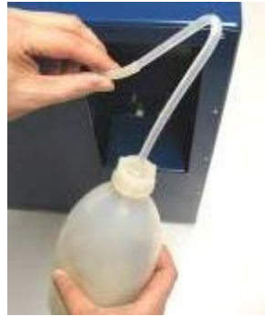
Fig. 4c Filling the U-tube
