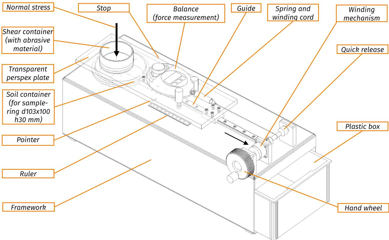
Schematic representation of surface shear apparatus
