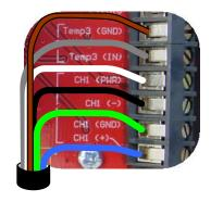
Using the DeltaLINK<sup>3</sup> logger software, configure channel 1 or 2 as sensor type **ML3** and channel 3 or 4 as an **ML3 Temperature** sensor. See also **GP1 Quick Start Guide** and the DeltaLINK on-line Help.
