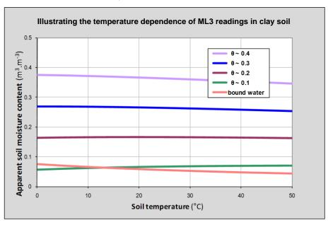
Note: ice has a quite different refractive index from water, so ML3 soil moisture readings cannot be interpreted reliably when inserted into soil below 0°C.
