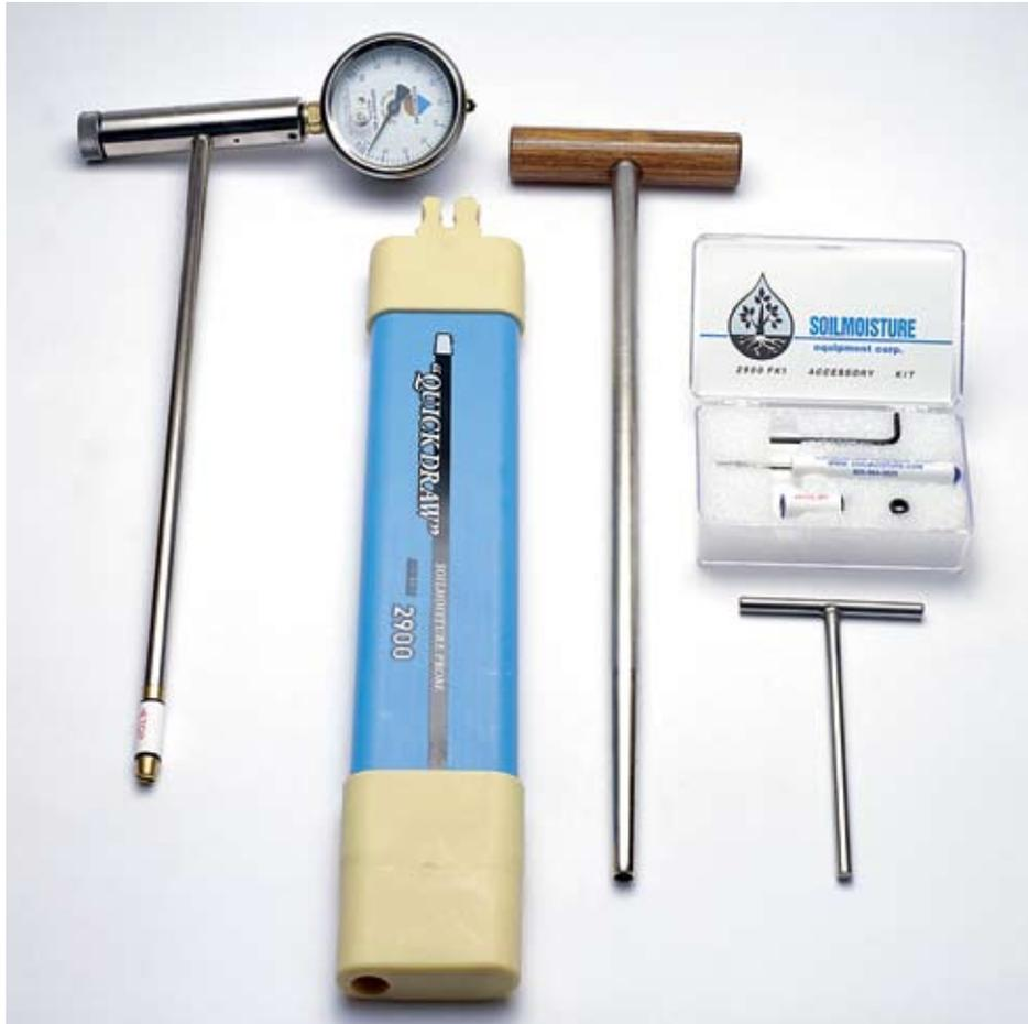
(Figure 1) - 14.04.05 Soilmoisture "Quick Draw" Probe
