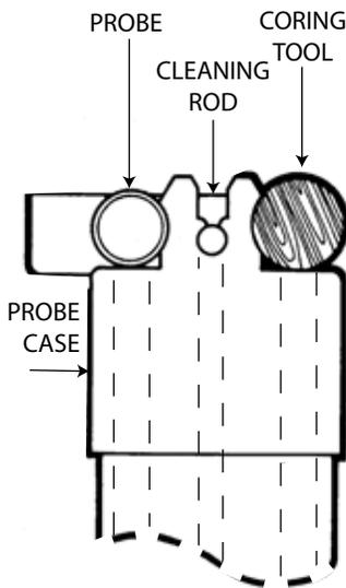
It is very important to keep the Probe in the side of the Carrying Case marked "PROBE" when it is not actually being inserted in the soil, because this side of the Carrying Case has a water storage reservoir at the bottom. During the "Initial Filling" operation, pictured and described on pages 7 through 10, you will fill the water storage reservoir. Thereafter, the sensing tip of the Probe will be kept moist.
