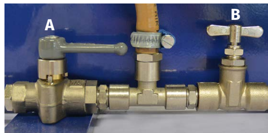
Fig. 17 Cock A is open, cock B is closed
