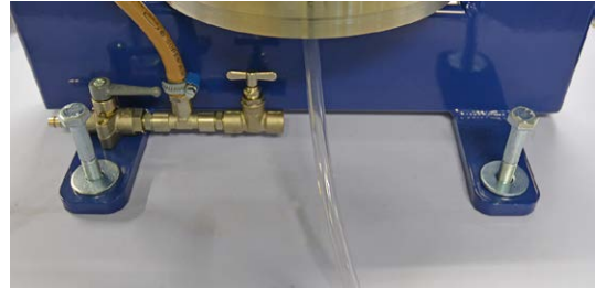
Fig. 1 Secure to a table with bolts
