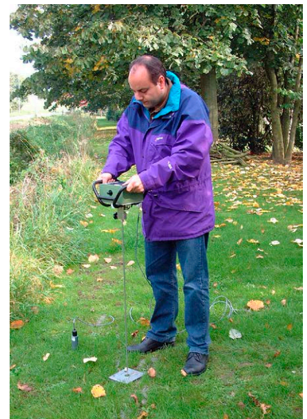
Measuring with the penetrometer
