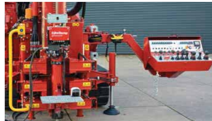
The Drill'n CPT mounted on the MidRotoSonic XL, ready for work.
