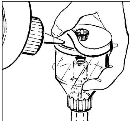
(Fig. 7a) Filling the Jet Fill Tensiometer
