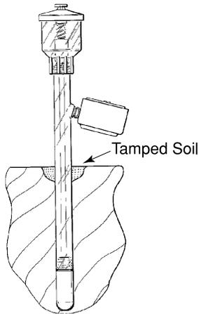
accept the tensiometer are always backfilled and the soil at the surface tamped tightly around the body tube. (Fig. 8b)
