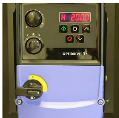
Fig. 8d Switch 3 set to 200 Hz
