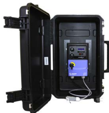
Fig. 7 Vertical installation of the converter
