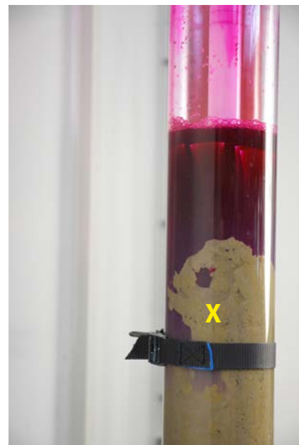
Detail product X permeable, test dye is leaking through bentonite when pumping.
