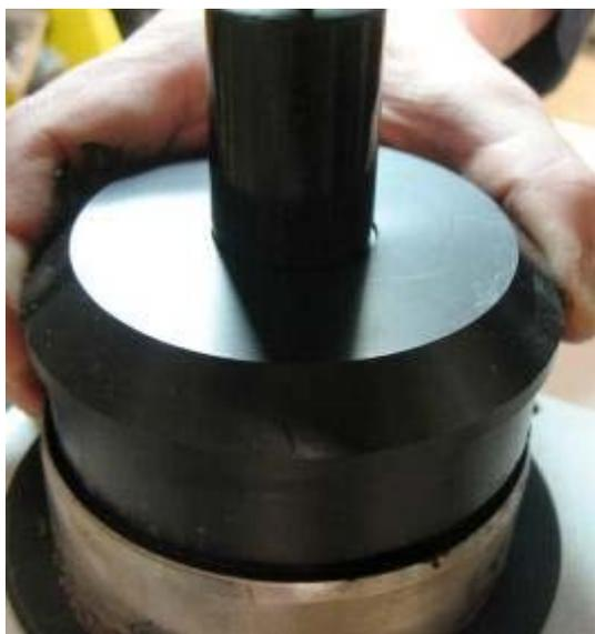
13 Remove the empty sample ring and the transfer ring.
