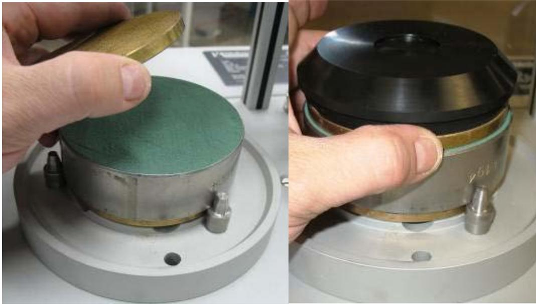
8 Lift the height sensor and place the rod and centre them carefully.
