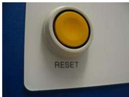
The button will be locked and a safe situation is secured. To recover turn the button clockwise to unlock and press the yellow button to continue.
