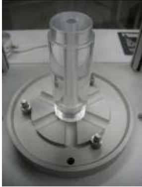
3 Place the sintered plate with the tensiometer spare hole on the sample chamber. Optional place a high flow filtration paper with tensiometer spare hole preventing smearing of the sintered plates.
