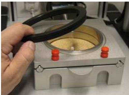
10 Place the sample with the tensiometer hole downwards on the transfer ring. Place the upper sintered plate optional using filtration paper.
